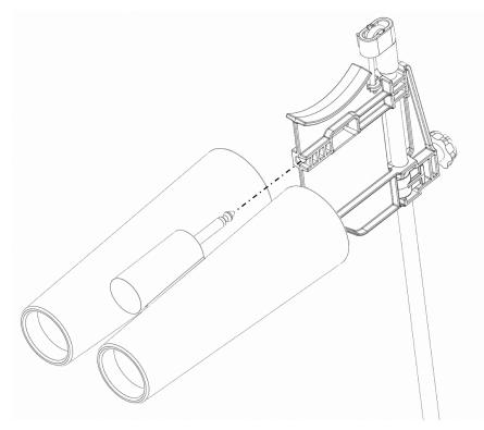
To use your long frame Kestrel system, always start by configuring the assembly for use by coupling the lower and upper legs together.
