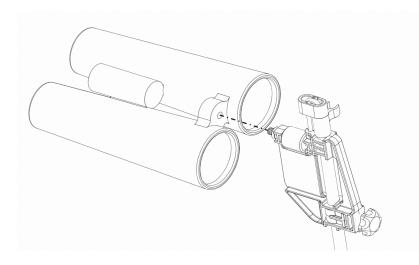
To use your short frame Kestrel system, always start by configuring the assembly for use by coupling the lower and upper legs together.
